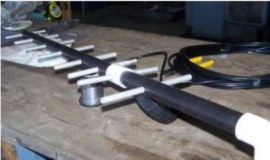
*It's a small antenna - widest aluminium element is 168mm*
