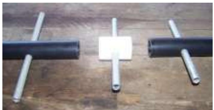
You're working with the critical dimensions between your Reflector and the Driven element when it's all back together that measurement must be 74mm. (see the table of specifications above)
